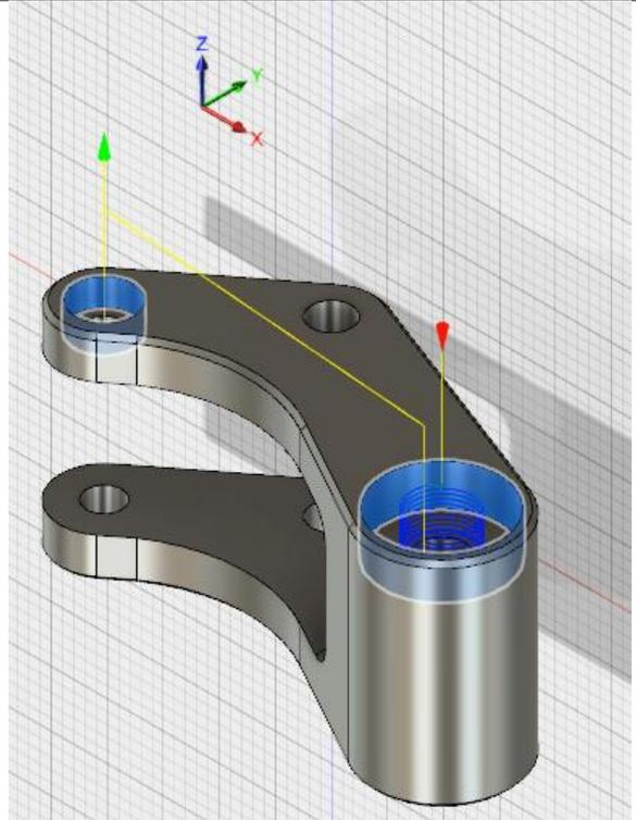
**Bore small holes:** Create a bore operation to machine the two small holes.
