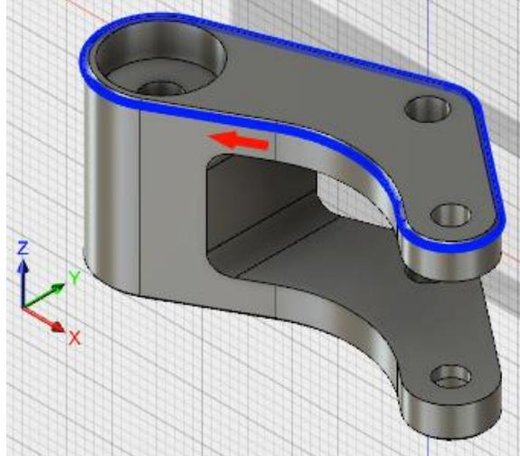
Step 4 – Set the chamfer tip offset
