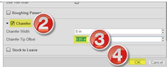
The center of a spinning tool is not rotating as it is at the center of rotation. Instead, it is just pushing material. By using a Tip Offset the tool slides down the chamfer and is cutting instead of pushing material resulting in a far better surface finish and avoiding the possibility of a step at the bottom of the chamfer.
