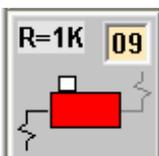
This device allows the user to connect to an 'Uno' pin either a 1 k-Ohm pull-up resistor to +5V, or a 1 k-Ohm pull-down resistor to ground. This lets you simulate electrical loads added to a real hardware device. By left-clicking on the slide switch *body* you can toggle your desired pull-up or pull-down selection. Using one, or several, of these devices would allow you to set a single (or multi)-bit "code" for your program to read and respond to.
