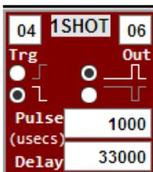
One possible use of this device is to simulate ultrasound ranging sensors that generate a range pulse in response to a triggering pulse. It can also be used wherever you wish to generate a pin input signal synchronized (after your chosen delay) to a pin output signal created by your program.
