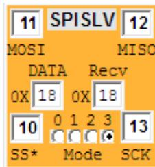
The device senses edge transitions on its **CLK** input according to the selected mode ( `'MODE0'`, `'MODE1'`, `'MODE2'`, or `'MODE3'` ), which must be chosen to match the programmed SPI mode of your program.
