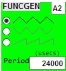
The period (in microseconds) can be set using the edit-box—the minimum allowed period is 100 microseconds. The waveform it creates can be chosen to be sinusoidal, triangular, or sawtooth (to create a square wave, use a 'PULSER' instead). At smaller periods, fewer samples per cycle are used to model the produced waveform (only 4 samples per cycle at period=100 usecs).
