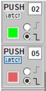
This 'I/O' device emulates a normally-open **momentary OR latching** single-pole, single-throw (SPST) push-button with a 10 k-ohm pull-up (or pull-down) resistor. If a rising-edge transition selection is chosen for the device, the push-button contacts will be wired between the device pin and +5V, with a 10 k-Ohm pull-down to ground. If a falling-edge transition is chosen for the device, the push-button contacts will be wired between the device pin and ground, with a 10 k-Ohm pull-up to +5V.
