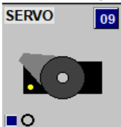
Your program must have an '`#include <Servo.h>`' line before declaring your Servo instance(s) *if you choose to use the Servo library functionality*, e.g. '`Servo.write()`', '`Servo.writeMicroseconds()`'. Alternatively, SERVO also responds to '`digitalWrite()`' "bit-banged" signals. Due to the internal implementation of UnoArduSim, you are limited to 6 'SERVO' devices.
