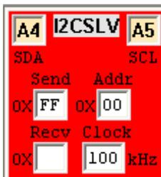
Your program must have an `'#include <Wire.h>'` line if you wish to use the functionality of the `'TwoWire'` library to interact with this device. Alternatively, you may choose to create your own bit-banged data and clock signals to drive this slave device.
