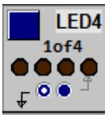
You can connect this row of 4 coloured LEDs between the chosen set of 'Uno' pins (each has a built-in hidden series 1 k-Ohm current-limiting resistor) to either ground or to +5V – this gives you the choice of having the LEDs light up when the connected 'Uno' pin is 'HIGH', or instead, when it is 'LOW'.
