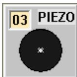
This device allows you to "listen" to signals on any chosen 'Uno' pin, and can be a useful adjunct to LEDs for debugging your program operation. You can also have a bit of fun playing ringtones by appropriately '`tone()`' and '`delay()`' calls (although there is no filtering of the rectangular waveform, so you will not hear "pure" notes) .
