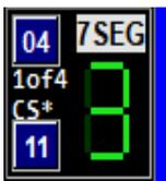
You can connect this 7-Segment Digit LED display to a chosen set of **four consecutive 'Uno' pins that give the hexadecimal code** for the desired displayed digit, ('0' through 'F'), and turn this digit on or off using the CS\* pin (active-LOW for ON).
