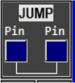
You can connect two 'Uno' pins together using this device (if any electrical conflict is detected when you fill in the second pin number, the chosen connection is disallowed, and that pin is disconnected).
