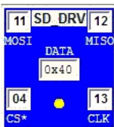
**A larger window displaying directories and files (and content) can be opened by double-clicking (or right-clicking) on the 'SD\_DRV' device.** All disk content is **loaded from** an **SD** sub-directory in the loaded program directory (if it exists) at '`SdVolume.init()`', **and is mirrored to** that same **SD** sub-directory on file '`close()`', '`remove()`', and on '`makeDir()`' and '`rmDir()`'.
