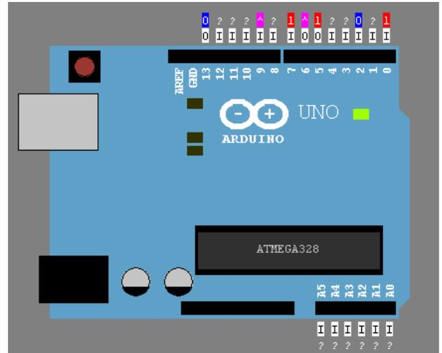
**Left-clicking** on any 'Uno' pin will open a **Pin Digital Waveforms** window that displays the past **one-second worth of digital-level activity** on that pin. You can click on other pins to add these to the Pin Digital Waveforms display (to a maximum of 4 waveforms at any one time).
