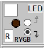
You can connect an LED between the chosen 'Uno' pin (through a built-in hidden series 1 k-Ohm current-limiting resistor) to either ground or to +5V – this gives you the choice of having the LED light up when the connected 'Uno' pin is 'HIGH', or instead, when it is 'LOW'.
