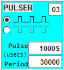
The period and pulse widths (in microseconds) can be set using edit-boxes—the minimum allowed period is 50 microseconds, and the minimum pulse width is 10 microseconds. The polarity can also be chosen: either positive leading-edge pulses (0 to 5V) or negative leading-edge pulses (5V to 0V).
