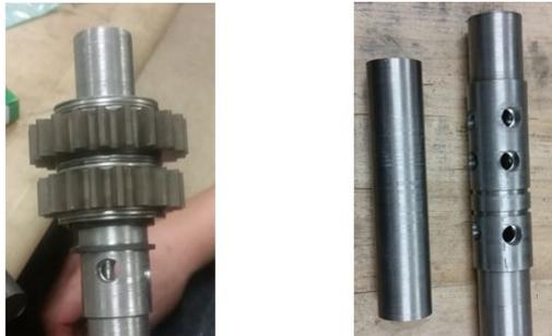
**Figure 10. Shafts and Ball Lock Gear Assembly**
