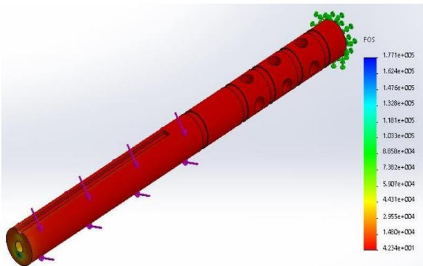
Figure 3. Factor of Safety of the Input Shaft
