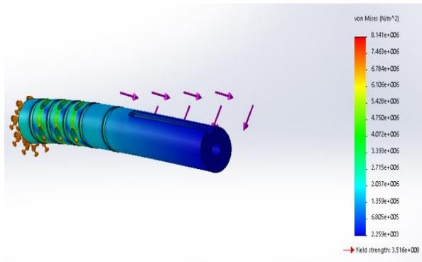
Figure 2. Stress on the Input Shaft
