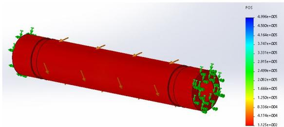
Figure 5. Factor of Safety of the 2<sup>nd</sup> Shaft
