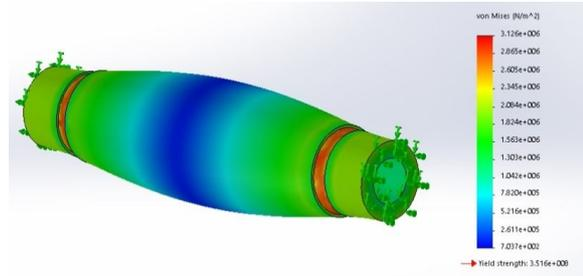
Figure 4. Stress on 2<sup>nd</sup> Shaft
