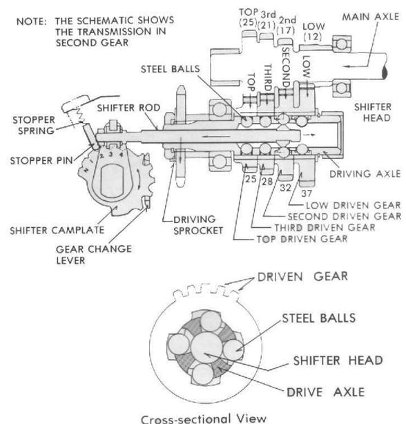
Figure 1. Ball Lock Shifter Mechanism [1]
